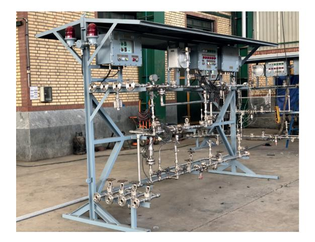
A reliable ignition system is one of the single most important aspects of a flare tip's safe operation. A flame front generator (FFG) ignition system is the most common method of lighting flare pilots. An FFG combines ignition fuel and compressed air in a mixing tee, and the air/fuel mixture flows through an ignition line to the pilot tip.
